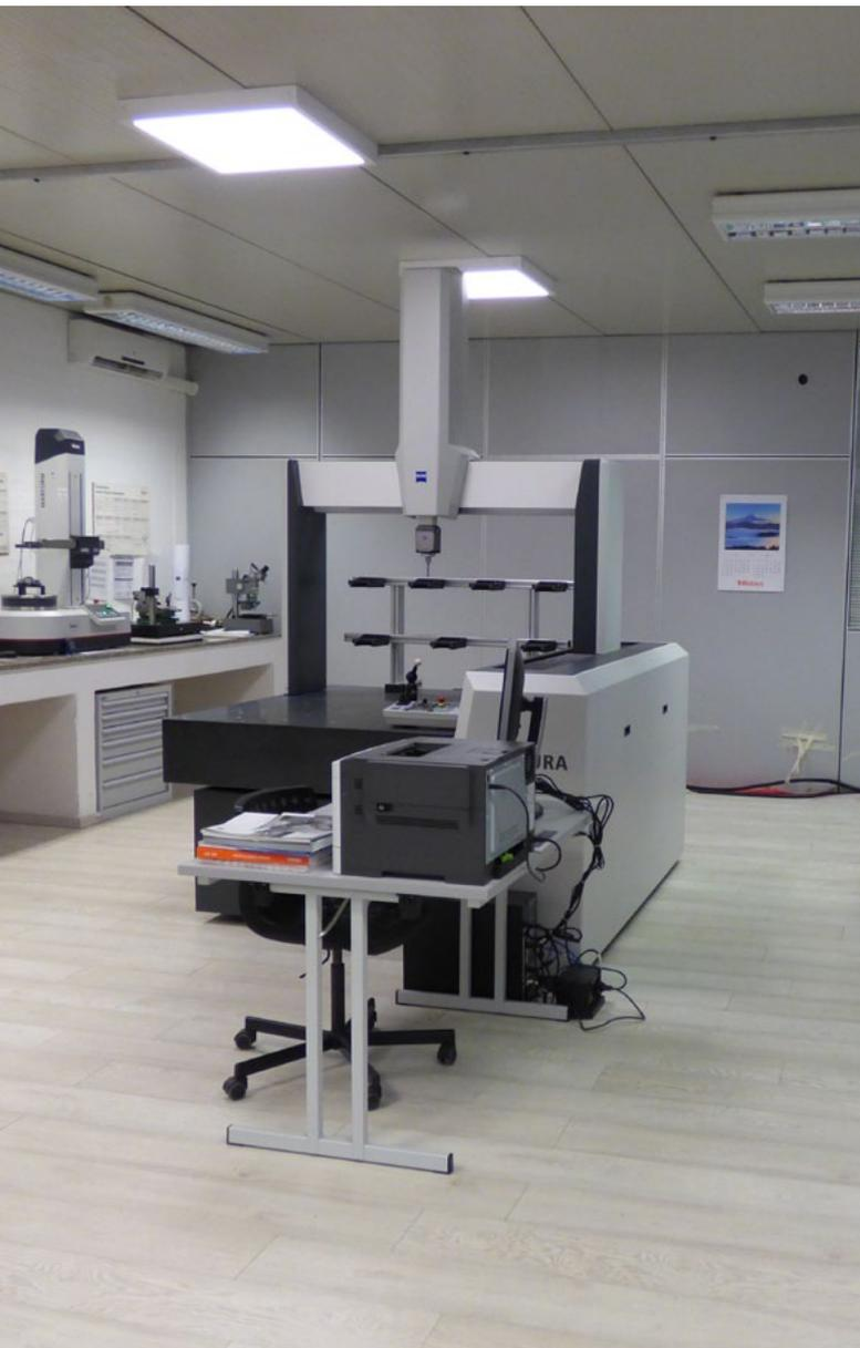
*The accuracy of the measurements is granted by the addition to active scanning of the VAST XT sensor which allows single-point measurements and which can complete practically any job: form and position measurements, curve and freeform measurements, and reverse engineering. The training attended by the person in charge of the lab room ensured that we will take the full advantage of the innovations offered by this machine in all the production aspects in OMC2.*
